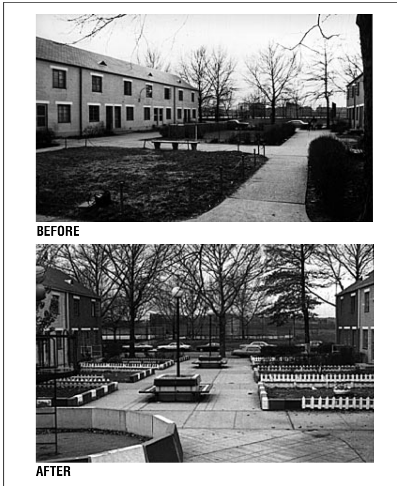
Figure III-15: Before and after photographs of an area of Clason Point. The original layout provided no grounds in the front of units for individual residents. In our site redesign, the central green area, which was largely neglected, was removed and residents were given their own front yards, which they quickly improved. A play node is shown at front left.
